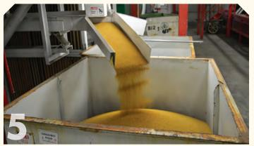
Many field lots are sufficiently cleaned for commercial sale after the inclined rollers. Lab testing of a representative sample will inform the operator whether more cleaning is needed. Each cleaning operation inevitably removes some viable seed along with the material targeted for removal. It's a judgment call whether to conduct more cleaning operations or to stop when the seed is within tolerance for "other crop" or weed seed and free of noxious weeds.
