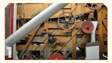
Seed is first run through a Clipper Cleaner, sort of like the back half of a combine, except that it's stationary. Just like a combine, air is blown up through a series of reciprocating sieves that are sized to exclude seeds larger than alfalfa. It also blows chaff and the lightest shriveled seed out of the good seed.
