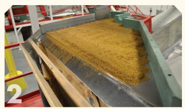
A gravity table is like an air hockey table lifted at a slight angle on one corner. It vibrates at about 250 shakes per minute. Seed moves across at a speed and distance related to its density. There are three "cuts" of seed coming over the edge . . . light or shriveled seed gravitates to one corner, while the heavy seed, including dirt or small stones, gravitates to the opposite corner. The middle "cut" is good seed.
