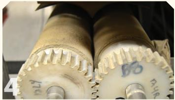
Rollers rotate up and away from the seed flowing down the channel in the middle where the rollers meet. Rollers are covered with a nappy, velvet-like fabric. Rough-coated weed seeds stick just enough to be pulled out and away from alfalfa seed as it flows down the channel due to its smooth seed coat.
