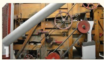
Seed is first run through a Clipper Cleaner, sort of like the back half of a combine, except that it's stationary. Just like a combine, air is blown up through a series of reciprocating sieves that are sized to exclude seeds larger than alfalfa. It also blows chaff and the lightest shriveled seed out of the good seed.
