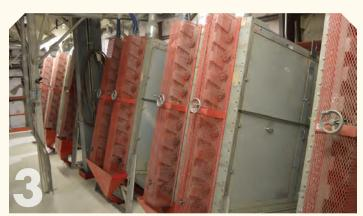
Since the clipper cleaner and the gravity table have already done most of the cleaning based on size and density, we turn to the principle of seed coat roughness to remove small weed seeds of many species. This bank of inclined velvet rolls removes weed seed of similar size and density to alfalfa seed. Rollers are inclined to allow seed introduced at the high end, to flow down the channel between the rollers and out the low end.
